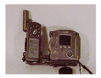
Fig. 2. Photo of DC260 camera with GPS receiver attached
